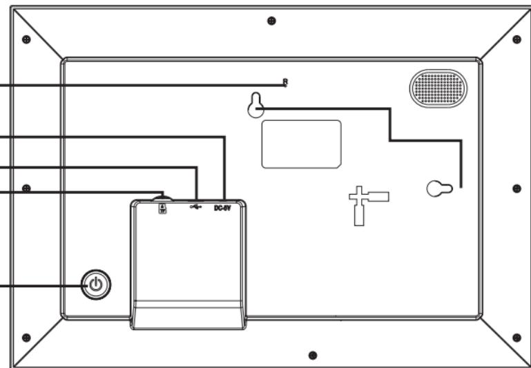
1. R- Using a needle or paper clip, press into the hole to power off the unit if the unit is frozen or has no response.
