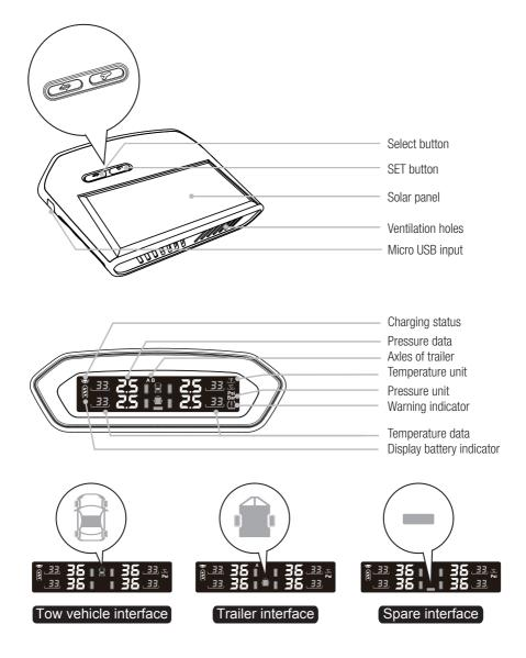
**Note:** The icon in the centre of the LCD display indicates the viewing interface.
