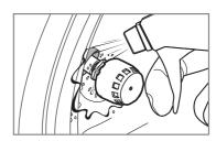
**Note:** Do not over-tighten sensors as this will effect the readings.
