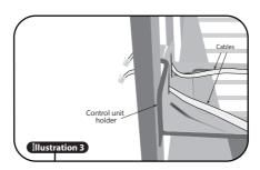
**PLEASE NOTE:** DO NOT ATTACH THE CONTROL UNIT TO THE TOP RAIL OF THE COT. DO NOT EXTEND CABLES IN ANYWAY.
