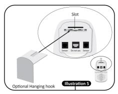
7. Press control unit holder or hanging hook firmly into slot in back of control unit as shown in illustration 5 and 6.
