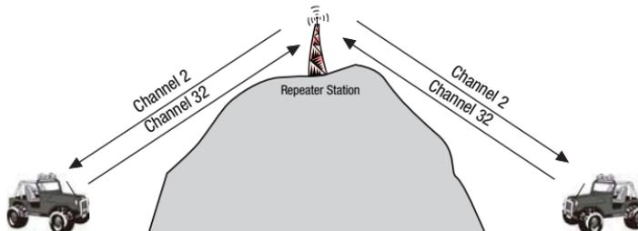
The Repeater Access function can be set (from channel 1 to 8 and 41 to 48) used by local repeater stations. When activated, your radio will receive the Repeater on its specific channel (all repeater outputs are on channel 1 to 8 and 41 to 48) but transmits to the repeater channel 31 through 38 and 71 through 78.
