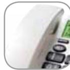
The TP170's amplified receiver provides 20dB of extra loud ear piece amplification for the hard of hearing. The phone contains an in-built inductive coupler which offers Hearing Aid users clearer sound. Simply switch the hearing aid to the 'T' setting to use this function.
