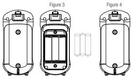
Caution: Observe the proper battery polarity orientation when installing batteries. Incorrect positioning can damage both the batteries and the unit.
