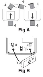
5. Position the mounting holes on the base of the phone over the two protruding screws on the wall plate. Gently push the phone flush against the wall plate then slide the phone downwards locking it into place.
