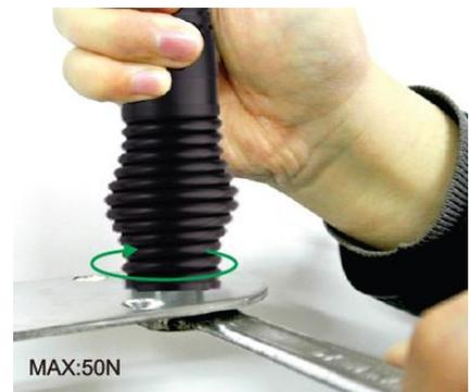
2. Install the fiberglass whip to the elevated feed by turning in a clockwise direction and hand tighten only MAX. 15N.
