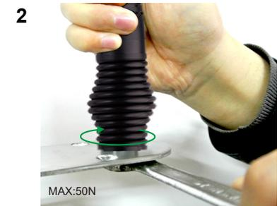
**To convert to a 1.4m 6dBi gain antenna**
