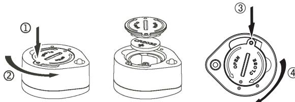
**CAUTION: This product is only to be used in water when assembled and operated in accordance with the instructions. If the battery cover is not fitted correctly then the seal will not be water proof and water will enter the product and result in damage.**
