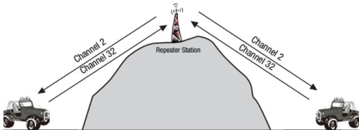
The Repeater Access function can be set (from channel 1 to 8 and 41 - 48) used by local repeater stations. When activated, your radio will receive the Repeater on its specific channel (all repeater output are
