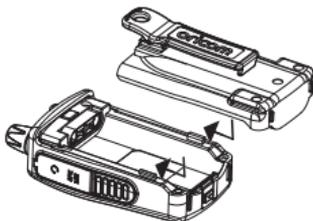
Remove Battery Pack - Push battery catch in direction of arrow and then slide the battery off.
