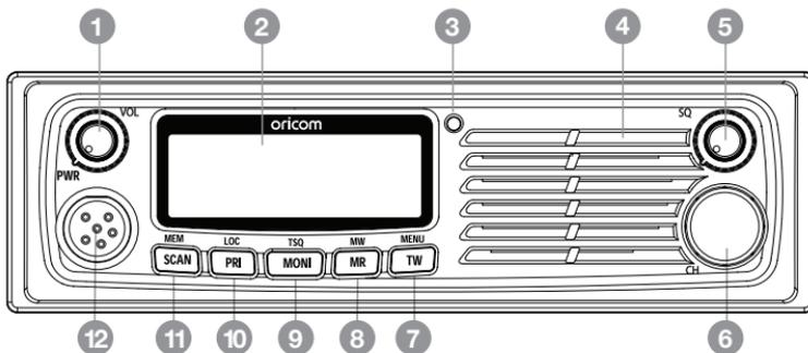
1. Rotary On/Off switch and Volume control
