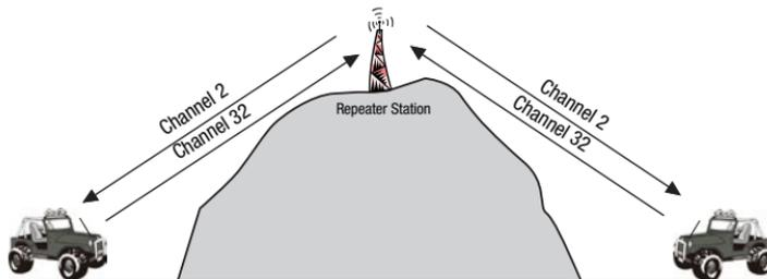
The Repeater Access function can be set (from channel 1 to 8 and 41 to 38) used by local repeater stations. When activated, your radio will receive the Repeater on its specific channel (all repeater outputs are on channel 1 to 8 and 41 to 48) but transmits to the repeater channel 31 through to 38 and 71 through to 78. (Factory default is set to On for all repeater channels).
