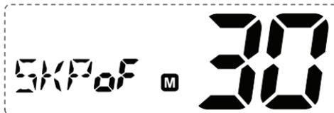
Note: To enable a skipped channel to scanning again, select the channel, then press and hold SCAN/MEM until SKPoF appears.
