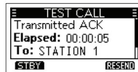
**NOTE:** If the Auto ACK function in "DSC Settings" is set to "Auto", the Test Acknowledgement call is automatically sent to the calling station when the call is received.
