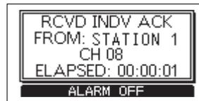
Press softkey **[ALARM OFF]** to turn OFF the alarm, the channel assigned in above step is automatically selected.
