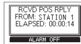
8. Press softkey [ **ALARM OFF** ] to turn OFF the alarm.
