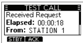
4. Press softkey [ **CALL** ] to send the Acknowledgement, "Transmitting Test Ack" is displayed.
