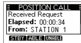
3. Press softkey [ **ABLE** ] to send an "Able to Comply" Acknowledgement, or press softkey [ **UNABLE** ] to send an "Unable to Comply" Acknowledgement.
