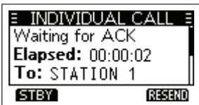
9. When you receive an Acknowledgement "Able to comply", an alarm sounds, the screen as below is displayed.
