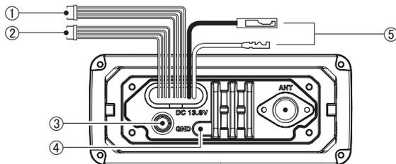
When connecting the external speaker, GPS, DC power supply, computer and navigation device by the rear panel cable end, cover the connectors and cables with rubber vulcanizing tape as below, to prevent water seeping into the radio.
