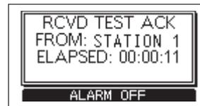
1. Press softkey [ **ALARM OFF** ] to turn OFF the alarm.
