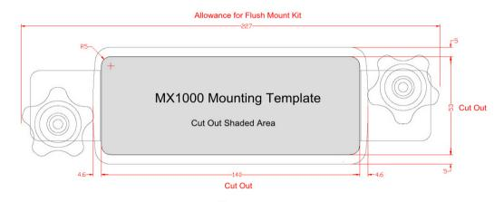
Allow 120mm from Radio Mounting Surface for Radio Depth
